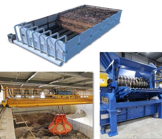
The first step of the organic line is constituted by the separation: dry, inert and other fractions are expelled by a centrifugal machine and fedback to the sorting line. The **organic** fluid obtained has a very good homogeneity which allow to reach a very high efficiency in the anaerobic digestion process.
